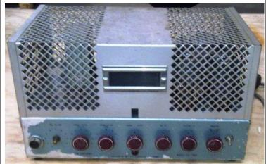
AWA 70W PA827 – retrofitted front panel socket and power switch.
