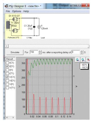
When modifying part values, PSUD2 will give an alert if a peak current limit is exceeded. Preferably cross check that the current limits are the same as in the datasheet.
