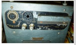
Older PA with hazardous terminals; hardened and crumbling rubberized wire insulation; & optional DC powering with vibrator. Circa mid 1940's Australian Sound Systems A13.
